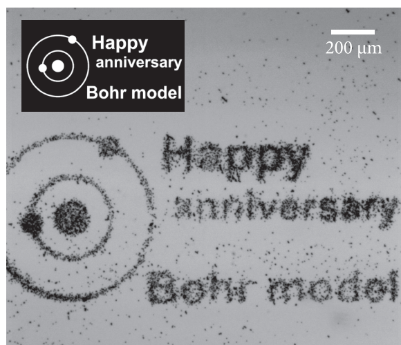
FIG. 3. Electrophoretic trapping on a z-cut lithium niobate crystal; the inset shows the desired amplitude-modulated image honoring Bohr's discovery of the shell model in 1913; the microscope image shows that charged particles adhere well to the previously illuminated regions without any anisotropy.
