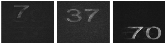
Fig. 2. Reconstructed analog data pages of a set of 70 pages that are recorded by means of 64 reference beams.
