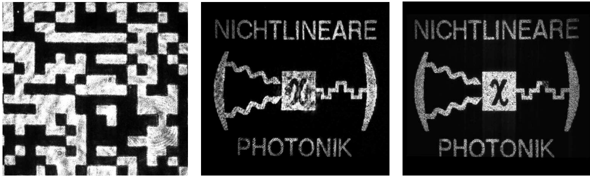
Fig. 3. Cut-out of a reconstructed digital (left) and analog (middle) data page that have been recorded in \text{Bi}_2\text{TeO}_5 using laser pulses and for comparison a analog hologram recorded in \text{LiNbO}_3 (right). The reconstruction of the data pages is performed by cw illumination of the same wavelength.
