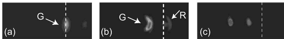
Fig. 17 Dynamics of soliton formation of a beam at \lambda = 532 nm (G) when guiding a probe beam at \lambda = 633 nm (R). The probe beam is located at the right side of the soliton due to a spatial frequency selection by using a prism in front of the recording CCD camera. The time interval between consecutive frames (a)–(c) is \Delta t = 3 s
