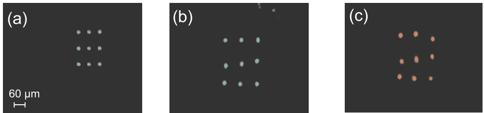
Fig. 19 Realization of a 3 \times 3 waveguide array induced by photorefractive solitons. (a) Front face of the crystal where the spot-array is imaged (distance between spots \delta x = 60 \mu\text{m} , \delta y = 80 \mu\text{m} ; intensity in every channels 110 nW; diameter of each spot 15 \mu\text{m} ). (b) Array of 9 focused solitons, (c) waveguiding in separate channels of the array of a probe beam at \lambda = 633 \text{ nm}
