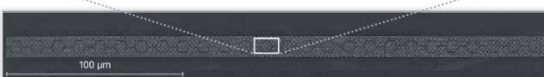
Write field stitching allows for direct milling of long waveguides with offsets on the 10 nm scale only.
