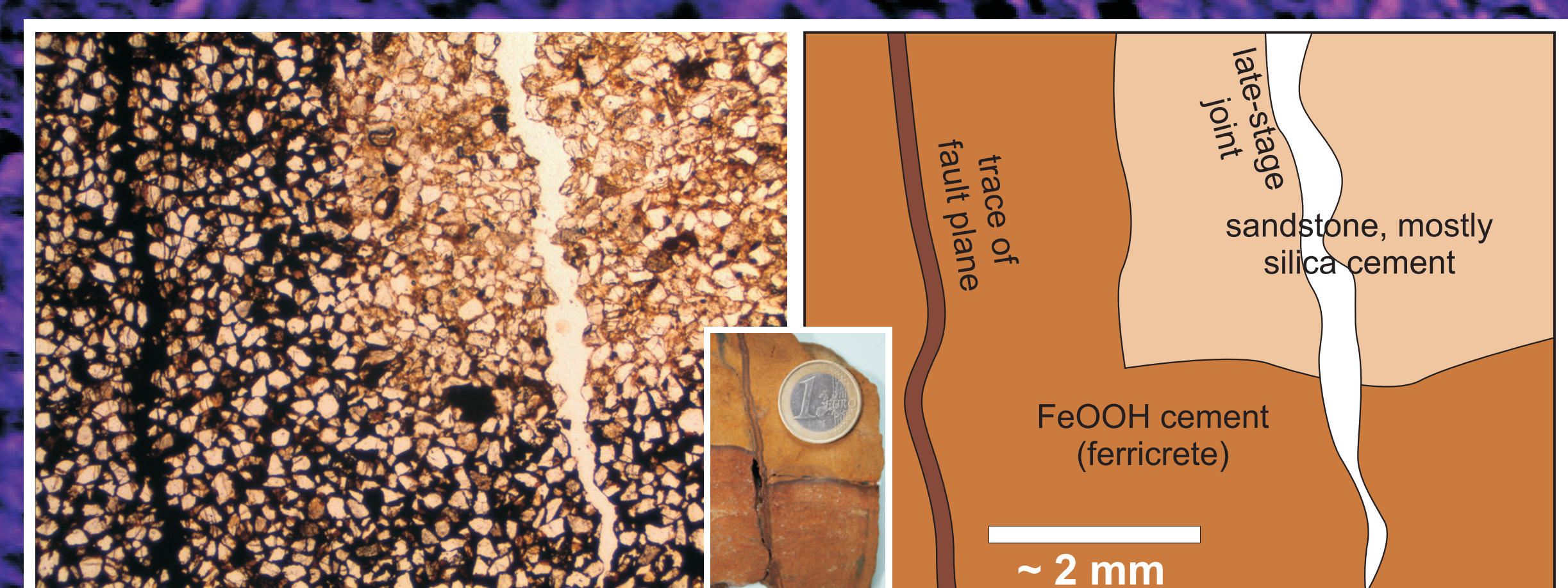
Fig 4 Thin section micrograph of an Fe impregnated small scale normal fault with a displacement of ~ 1 cm. Note the cracked quartz grains close to the fault surface.
