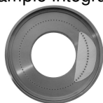
Sample on impactor stage equipped with Tedlar® foil and quartz fibre filter on top
