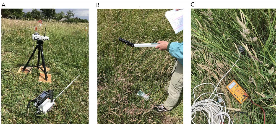
Fig. 7: Photographs of the three methods to measure the LAI with field instrumentation: A) SunScan S11, B) LAI-2200C, C) Pyranometer (type CMP3)
