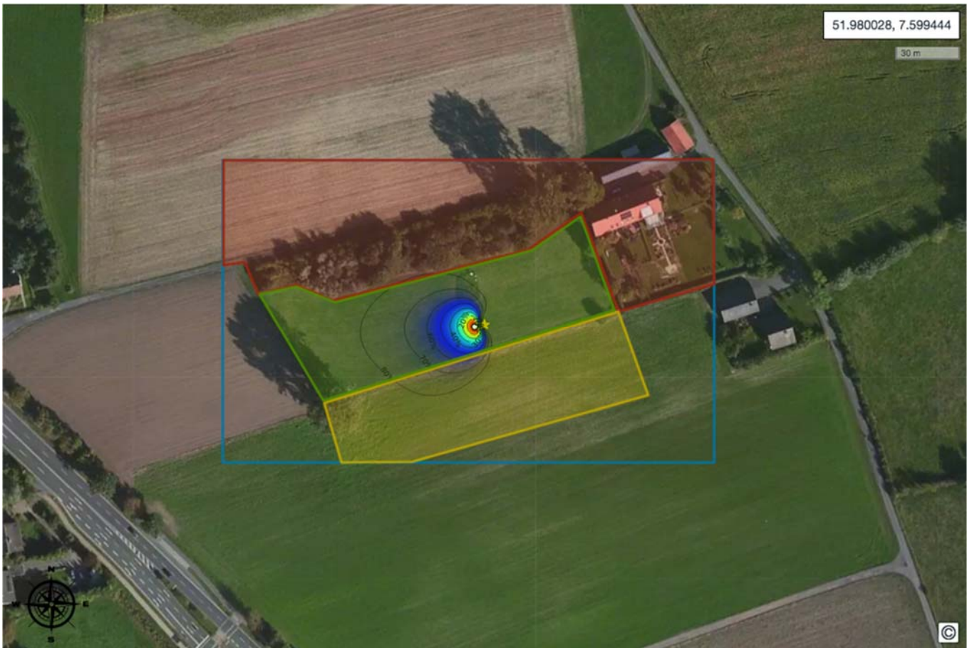
Fig. 2: Footprint representing field of view during period 1 (shades representing areas of uniform surface characteristics; Satellite Imagery: Mapbox)
