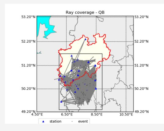
All rays (both P and S phase) used as input are plotted. Final contribution of rays depends on quality at each frequency range required for processing method
