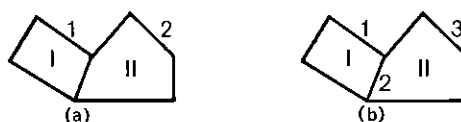
Fig. 8 Storage methods of borderlines: a: polygon mode b: segment mode In a the area I is described by the polygon 1; in b I is described by the segments 1 and 2.
