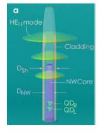
InP nanowires act as antennas for photons emitted by InAsP quantum dot insertions in their core. The size and spacing of the dots that form a molecule can be controlled very accurately.
