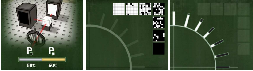
FIG. 2: Left: At the polarizing beam splitter, the polarization state of the photon |\Omega_{\text{Polarisation}}\rangle = e^{i\omega t} \cos\theta|\hat{V}\rangle - e^{i\omega t} \sin\theta|\hat{H}\rangle is split into the transmitted component \langle\hat{H}|\Omega_{\text{Polarisation}}\rangle = -e^{i\omega t} \sin\theta and the reflected component \langle\hat{V}|\Omega_{\text{Polarisation}}\rangle = e^{i\omega t} \cos\theta . Here, |\hat{H}\rangle and |\hat{V}\rangle are the horizontal and vertical axis at the polarizing beam splitter. Middle: Measured transmission and reflection results for single photons, visualized as random black-and-white patterns. At the rotatable half wave plate the angle \theta is increased in intervals of \theta = \pi/12 relative to the horizontal axis |\hat{H}\rangle . Right: Resulting transmission and reflection probabilities p_{\hat{H}}(\theta) = \cos^2\theta and p_{\hat{V}}(\theta) = \sin^2\theta .
