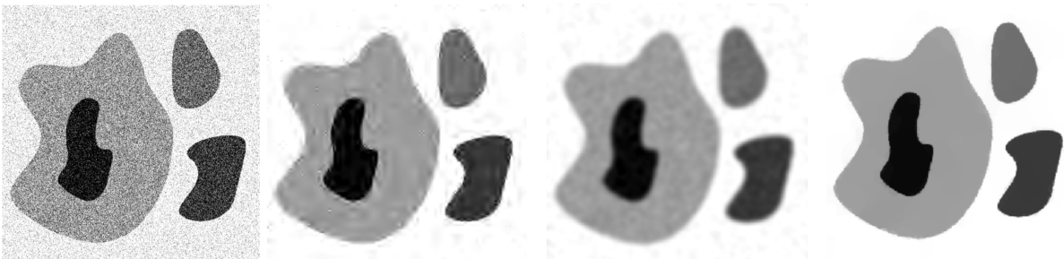
Figure 7: Original image from with noise (Picture 1), processed using wavelet algorithm (Picture 2), Gaussian filter (Picture 3), and TV regularization (Picture 4).
