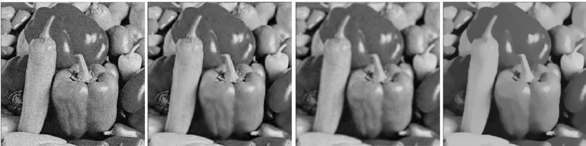
Figure 5: Original image from [21] with noise (Picture 1), processed using wavelet algorithm (Picture 2), Gaussian filter (Picture 3), and TV regularization (Picture 4).
