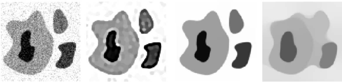
Figure 8: Blurred image with noise, subsampled on a 100 x 100 grid (Picture 1), TV-reconstructed with \lambda = 0.01 (Picture 2), TV-reconstructed with \lambda = 0.2 (Picture 3), and TV-reconstructed with \lambda = 1.5 (Picture 4).
