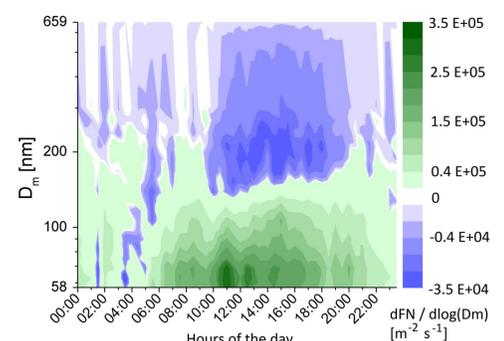
Fig. 4: Contour plot of mean daily number fluxes (normalized). Y-axis in log scale.
