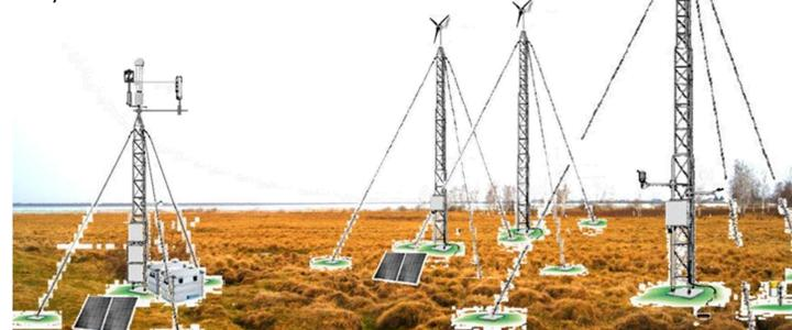
Fig. 6: Sketch of the measurement installation.
