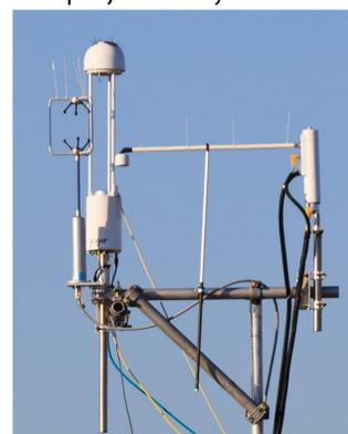
Fig. 5: Measurement setup of the eddy covariance stations.
