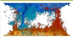
Volume rendering of a temperature field at parameters  $R_a = 10^9$ Pr = 1 and  $\Gamma = 2$ . Red corresponds to hot, blue to cold parts of the fluid. The volume rendering is done with the free volume rendering engine Voreen [8], developed at the University of Münster.
