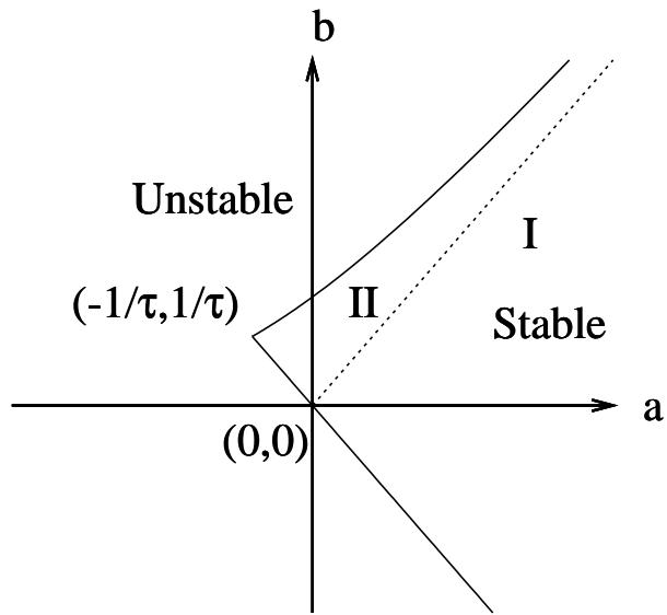
**Figure 1.** Parametric stability diagram for the linear SDDE (2). The stable region is defined by the intersection between two solid lines: one is the stationary bifurcation line  $a = -b$  (lower line), the second is obtained from the parametric equations Eq. (17) (upper line). Subset I determines the stable region given by  $a > |b|$  where the critical delay  $\tau_c$  does not exist and subset II determines the stable region satisfy both  $b > |a|$  and  $\tau < \tau_c$ .
