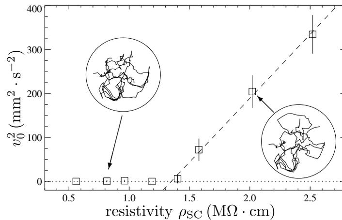
**Figure 4.** Experimental results for the square of the intrinsic speed  $v_0$  as a function of the bifurcation parameter  $\rho_{SC}$  and exemplary trajectories for parameters below and above the bifurcation point with circles denoting the active discharge area. Parameters:  $U_0 = 3700$  V,  $R_0 = 10$  M $\Omega$ ,  $p = 286$  mbar,  $T = 105$  K,  $d = 750$   $\mu$ m,  $t_{exp} = 0.02$  s, with  $I = 107$   $\mu$ A.
