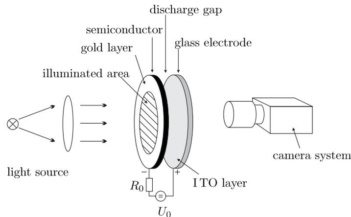
**Figure 1.** Schematic plot of the experimental set-up. It mainly consists of a high ohmic semiconductor electrode, contacted with a gold layer, a discharge gap filled with nitrogen and a transparent ITO electrode. The resistivity of the semiconductor is controlled by homogeneous illumination with visible light. The maximum global current of the discharge is restricted due to a series resistor  $R_0$ . The discharge can be observed with a CCD camera system through the transparent ITO electrode.
