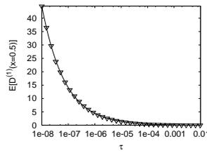
**Fig. 2.** Error of drift estimate as function of time increment  $\tau$  (triangles). A divergent behaviour for  $\tau \rightarrow 0$  is evident. The solid line represents the best fit  $f(\tau) = 0.0045/\sqrt{\tau}$ .
