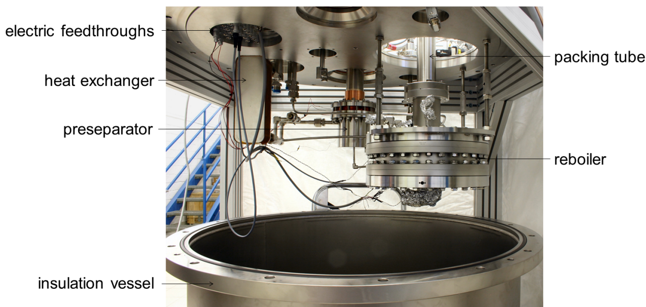
Figure 5.3: An insight into the bottom insulation vessel is shown. It contains the heat exchanger and the preseparator which are used to cool down and liquefy the xenon as well as the reboiler that is used to evaporate the xenon during the distillation process.
