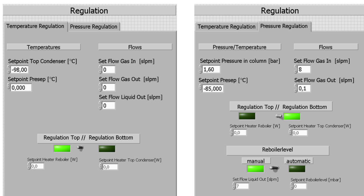
Figure 5.16: The temperature regulation (left), using the temperature measured by the silicon diode at the top as process variable, and the pressure regulation (right), using the pressure inside the column tube as process variable, are shown. In both cases, the control variable is either given by the heat cartridges at the top (Regulation Top), while the heater at the bottom can be controlled manually, or vice versa (Regulation Bottom). In both cases, all three flows can be controlled as well as the temperature in the preseparator. In addition, an automated regulation for the liquid level in the reboiler was implemented for pressure regulation.
