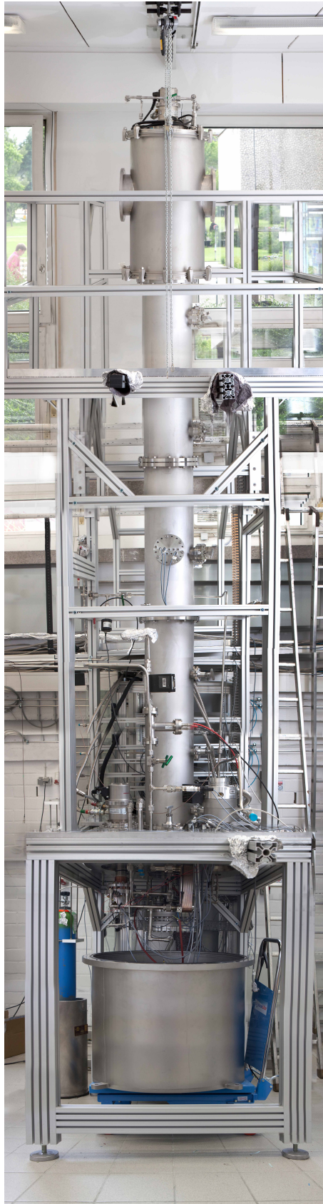
Figure 4.5: Picture of the 5 m distillation column being prepared for the XENON1T experiment. The insulation vacuum vessel is lowered, providing a clear view on the reboiler.
