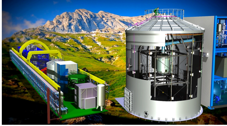
Figure 3.5: Schematic illustration of the XENON1T detector and its position inside the Hall B at LNGS. As seen on the right part the cryostat with the embedded TPC is surrounded by a 9.6 m diameter water tank, while the supporting structure is outsourced to the structure building, directly next to it. Figure in courtesy of the XENON collaboration.
