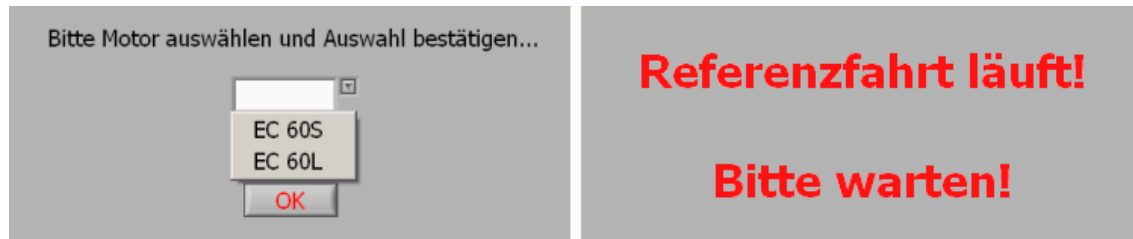
Figure 5.16.: Pop-up windows inform the user of the current step. Left: The user chooses a type of motor to be initialized. Right: The user has to stand by during homing mode.
