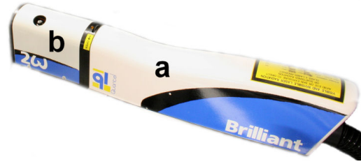
Figure 6.2.: The ablation laser consists of an optical head (a), a second harmonics generator module (b) and a power supply and cooling group cabinet (not shown) to which the optical head is connected by an umbilical.
