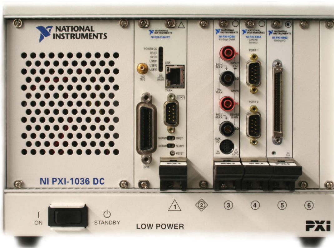
Figure 5.12.: The PXI-system consists of a chassis that holds several modules. The real-time controller module (slot 1), the CAN controller module (slot 4) and the timing- and digital-I/O module (slot 5) are required for the test setup.
