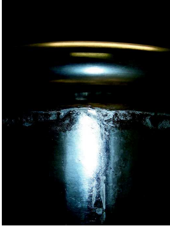
Figure 6.22: Welding seam at the pre-spectrometer ground electrode
