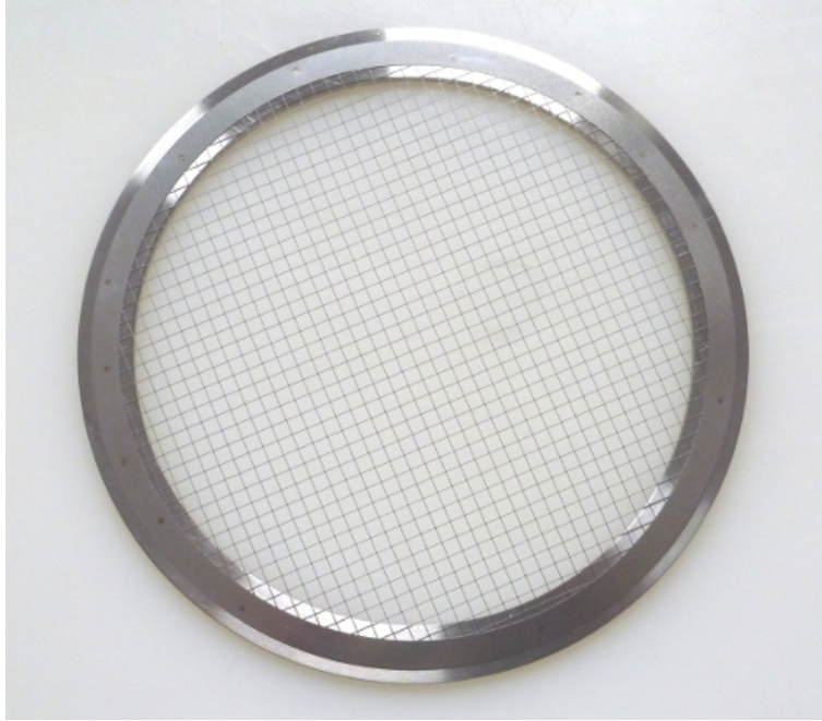
Figure 4.2.: Custom made mesh for the Münster TPC welded on a stainless steel ring for test purposes. This connection can be created with little effort, but high quality.
