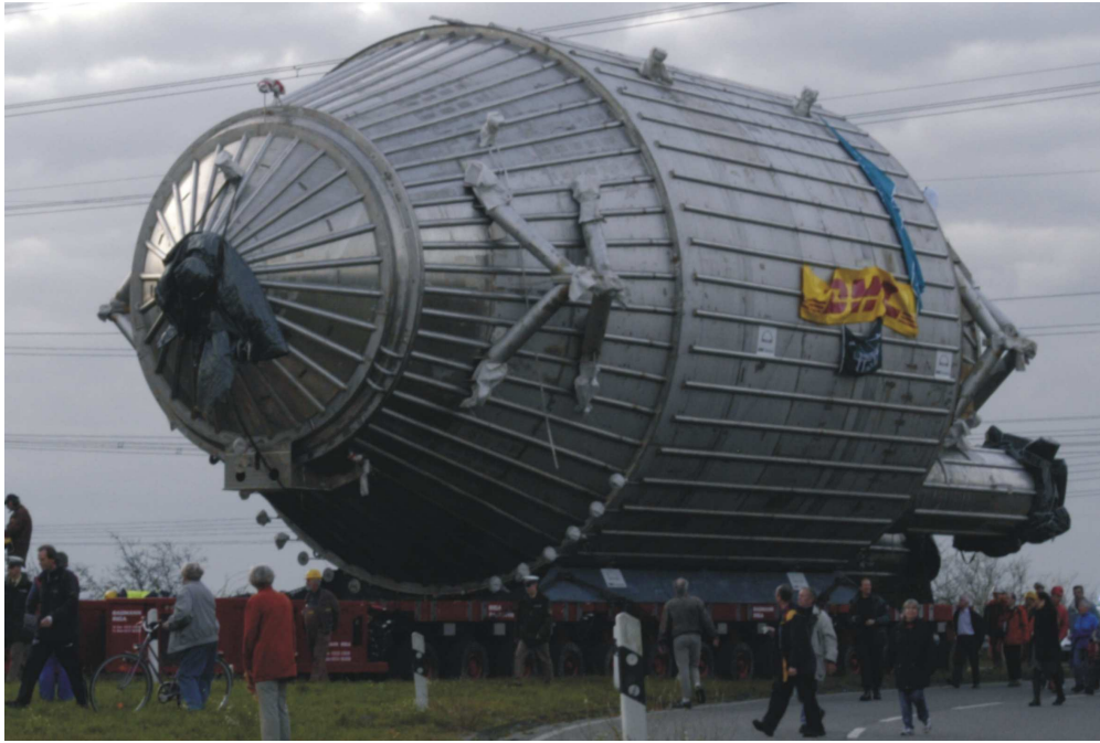
Figure 1.3.: Photo of the KATRIN main spectrometer during transport to FZK.
