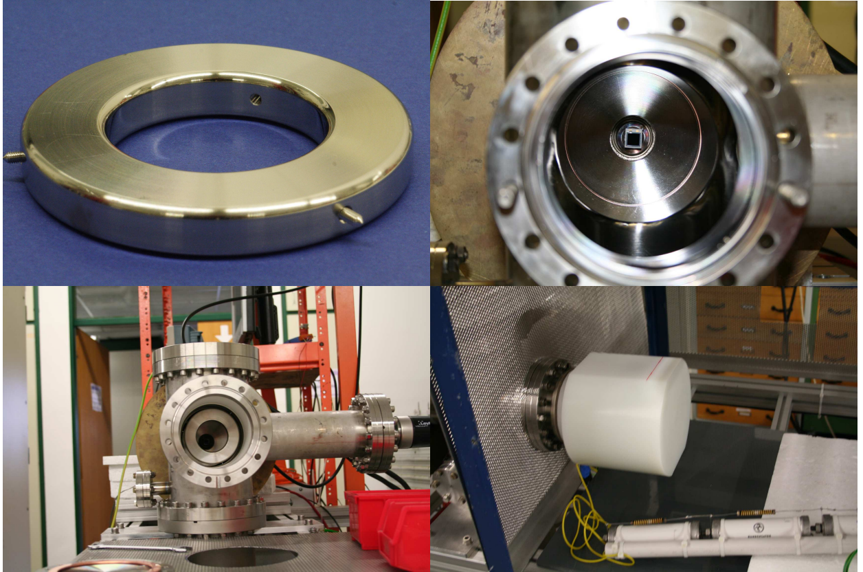
Figure 4.4.: Top left: The ring electrode which grounds the electric field and ensures a smooth field, before mounting in the isolator flange. Top right: View of the interior of the vacuum chamber cross piece. The detector is visible in the back. Bottom left: View of the vacuum chamber along the z-axis with the isolator tube attached. The electrode is visible in the isolator section. Bottom right: View of the isolator with the PVC endcap mounted, the red line denotes the inner extent of the electrode. Also visible are the HV-capacitors for the voltage smoothing.
