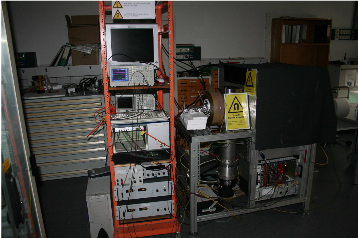
Figure 4.7.: View of the setup, as used in the last four runs. The cloth covering in place over the high-voltage cage which ensures no light enters the vacuum chamber was not removed for this photo.
