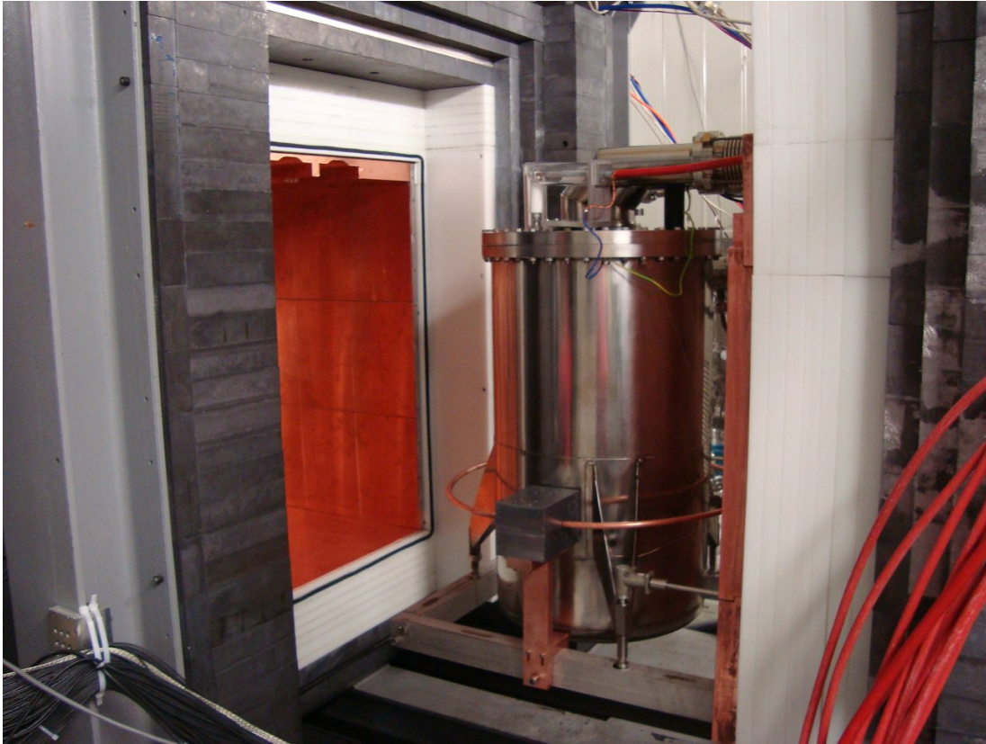
Figure 3.5.: The XENON100 detector enclosed in the titanium vessel with open shield structure comprising copper, PTFE and lead blocks. The circular copper pipe around the detector enables insertion of calibration sources [Apr10c].
