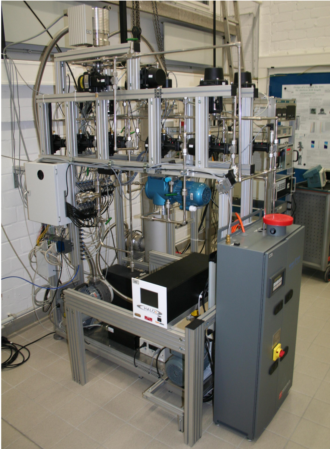
Figure 3.8.: Prototype of gas system schematically shown in figure 3.7. The SAES getter is housed in the gray board which can be seen on the right hand side. Behind the getter inside a black box the Halo+ Trace Gas Analyzer is located. The blue KNF pump for gas circulation is visible centered underneath the gas rack. The pneumatic bellow valves are housed inside the black boxes at the top of the gas rack. The turbo molecular pump is placed precipitately on top of the gas rack in the upper left corner.
