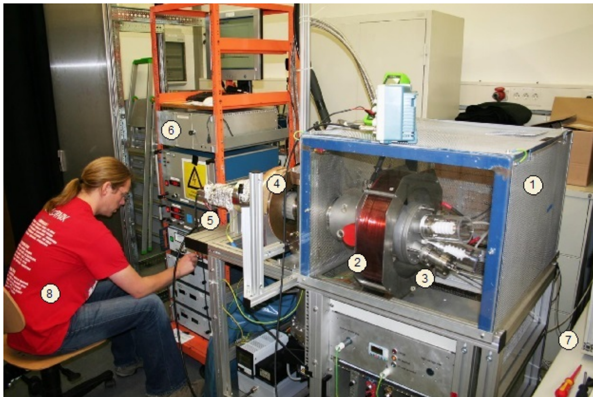
Figure 6: The eGun test setup. (1) Grounded HV-cage, (2) eGun magnet/ Hillen-coil, (3) eGun flange, (4) detector magnet/ Baumeister-coil, (5) detector, (6) rack with power supplies and DAQ computer, (7) optical fibre coming from the laser box, (8) Ph.D. student Michael Zacher. [Pos11]
