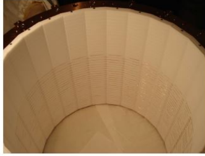
Figure 3.2: The PTFE covering of the XENON100 detector. Credits: XENON Dark Matter Project
