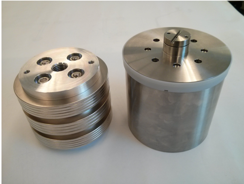
Figure 17: Inner piston magnets with container, made by Stanford University
