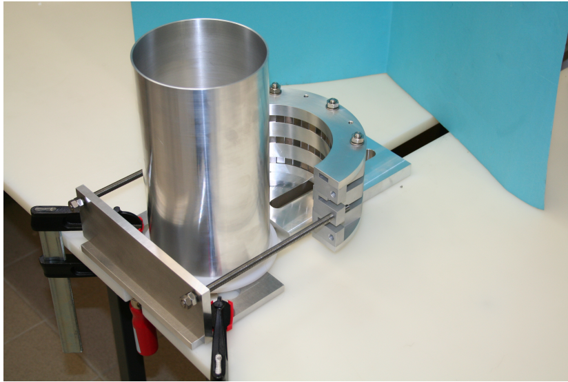
Figure 22: The first half ring can slide towards the tube by turning the two double nuts at the vertical plate counterclockwise.
