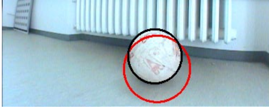
Fig. 5. The white non-RoboCup ball is precisely segmented in front of a white-grey background. This is hardly possible with color labeling. (red: initialization, black: estimated ball contour)
