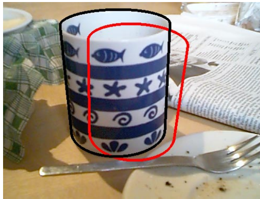
Fig. 10. An example of a cylindrical mug: the cylinder contour fitted to the image data matches the mug's contour. The estimated parameters of the contour are the five pose parameters of the cylinder. (red: initial contour, black: estimated contour)
