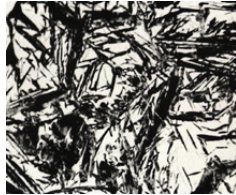
hard and brittle martensite high volume
