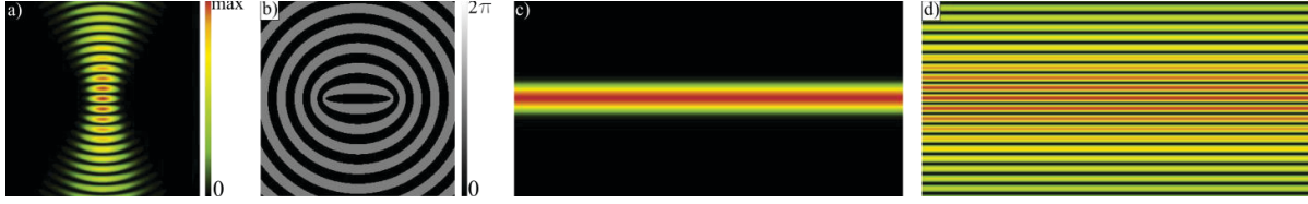
Figure 3 Nondiffracting even Mathieu beam of zeroth order: (a) transverse (xy-) intensity, (b) transverse phase, (c) xz-intensity, and (d) yz-intensity distribution.
