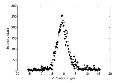
Figure 2: Z-Cut of beads (diameter 1  $\mu$ m) as seen in the Dynamic Phase-Contrast microscope. Note the symmetry of the response function as compared to the asymmetric response in Fig.1
