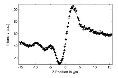
**Figure 1:** Z-Cut of beads (diameter 1  $\mu$ m) as seen with partially coherent illumination ( $\lambda = 532$  nm). The spatial coherence of the laser light is eliminated with a rotating diffuser.
