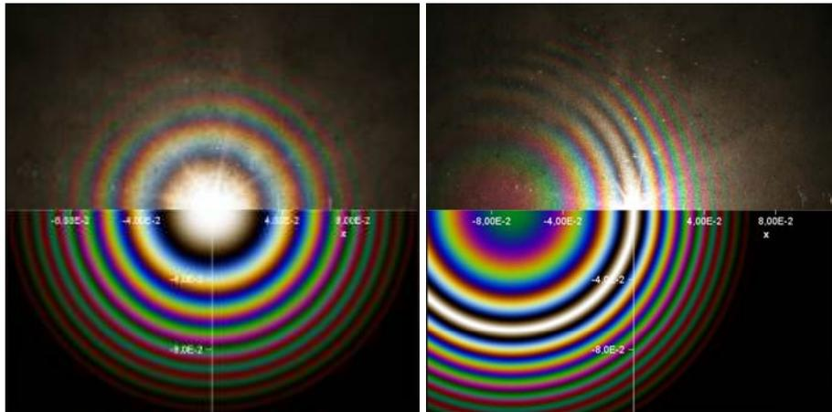
Figure 8 Concentric (left) and eccentric (right) interference rings. Upper part: Photograph of an impure mirror. Lower part: Representation of the corresponding model calculation.
