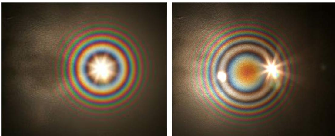
Fig. 4 Coloured rings produced with the setup shown in figure 3. On the left: Concentric rings. On the right: By slightly distorting the mirror eccentric rings appear.
