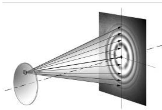
Fig. 5: Each element of the mirror produces a similar elementary ring system
