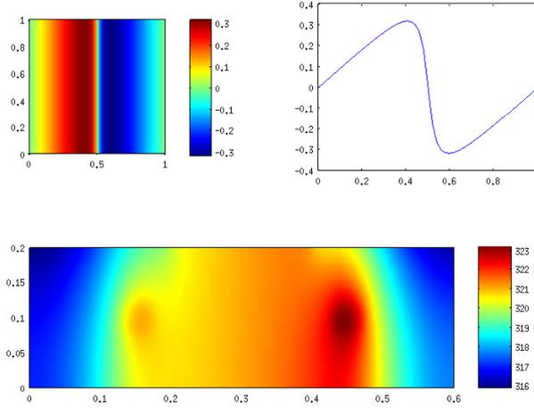
FIGURE 2. Example of a solution of the test problem for  $\mu = (0.9112, 0.0062)$ . Top left:  $\chi_H^1(\mu)$ , top right: cross-section plot of  $\chi_H^1(\mu)$  in  $y_1$ -direction; bottom:  $u_H^0(\mu)$ . The effective diffusion tensor is  $\mathcal{B}_h^0(\mu) = \text{diag}(0.069, 0.429)$ .
