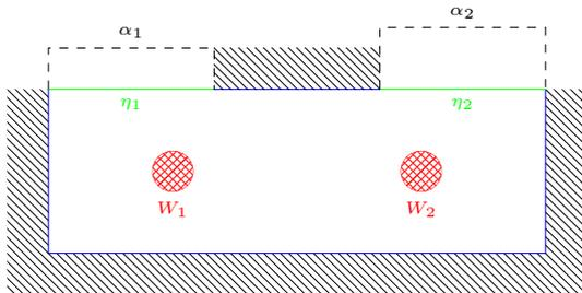
FIGURE 1. Geometry of the model problem: Two heat sources (red), no flow (blue) and Robin (green) boundary conditions. The head transfer coefficients and surrounding temperatures are  $\eta_1 = 0.3$ ,  $\eta_2 = 0.4$  resp.  $\alpha_1 = \alpha_2 = 300$ .
